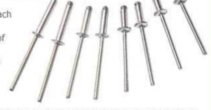
The rivet assembly is inserted into a hole drilled through the parts to be joined and a specially designed tool is used to draw the mandrel into the rivet. This expands the blind end of the rivet and then the mandrel snaps off. These types of blind rivets have non-locking mandrels and are sometimes avoided for critical structural joints because the mandrels may fall out, due to vibration or other reasons, leaving a hollow rivet that has a lower load-carrying capability than solid rivets.
