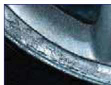
Curbside Rash & Scuffs
