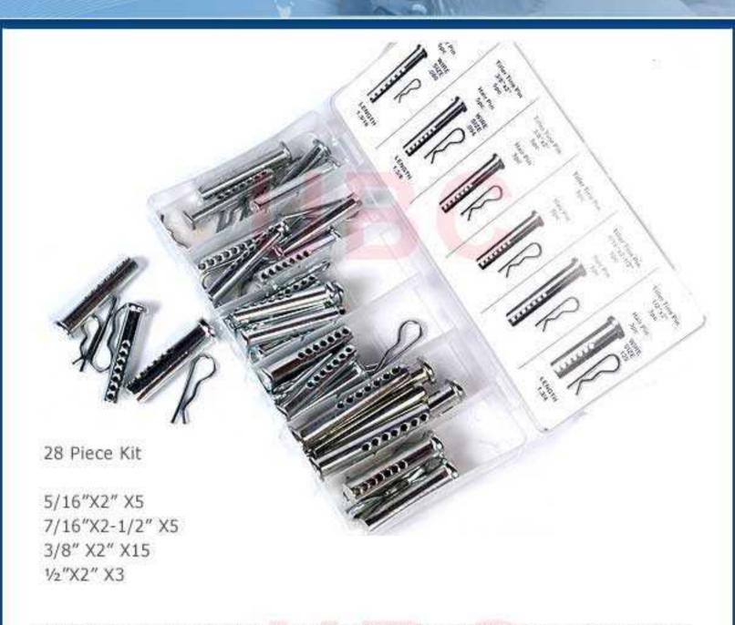
Clevis hitch pin kit 28 piece. A clevis fastener is a three-piece fastener system consisting of a clevis, clevis pin, and tang. The clevis is a U-shaped piece that has holes at the end of the prongs to accept the clevis pin. The clevis pin is similar to a bolt, but is only partially threaded or unthreaded with a cross-hole for a split pin. The tang is a piece that fits in the space within the clevis and is held in place by the clevis pin.
